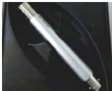
传声器 (采集噪音信号) Microphone (Collecting noise signals)
